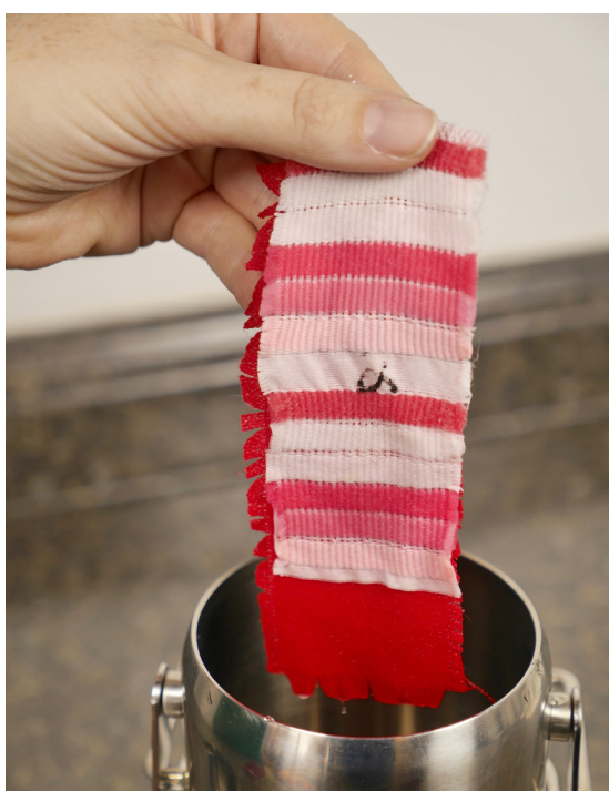
Stained Multifiber from Rotawash Container
